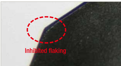
1. Less wear and flaking on the rake surface
